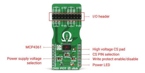
DIGI POT 5 click has one 2x10 pin standard, 2.54mm pitch header used to connect the four potentiometer terminals. There are three SMD jumpers onboard:
