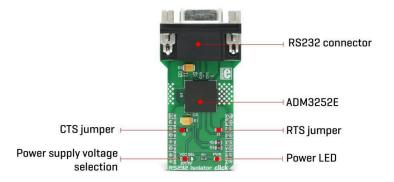
Besides the UART RX and TX lines, the click also supports the hardware flow control via the CTS and RTS lines. One of the two existing channels is used for the UART data communication itself, while the other channel is used for the hardware flow control lines. The usage of the control lines is not always mandatory, so the lines can be disconnected from the mikroBUS if needed, by unsoldering the SMD jumpers labeled as J1 and J2.
