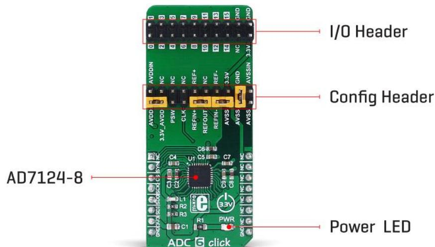
The signal routing in the AD7124-8 ADC is done via the internal multiplexer section, which is used to reduce the number of IC pins, yet allowing all of the functions to be used on the existing pins. On a top of these pins, there are four more GPIO pins that can be used for various tasks, including control of the multiplexer unit. Since the multiplexer is integrated into the chip, the conversion process stays synchronized with the changes made to the pin configuration.
