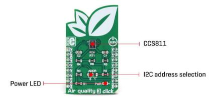
Because of the nature of the MOX sensors, the CCS811 sensitivity will change over the time, especially in early life use. The internal sensor resistance will change the most for the first 48 hours of operation. So, to achieve a proper operation of this sensor, it has to be calibrated during several different phases of its lifecycle. Since this step is important for achieving accurate IAQ results, it is strongly advised to be carefully studied from the CCS811 datasheet.
