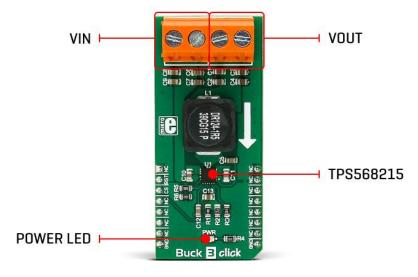
The onboard voltage divider connected to the MODE pin of the IC is used to set the device to work with the fixed PWM frequency of 800kHz, DCM/Eco-mode<sup>TM</sup> for light loads, and to set the limiting current to about 7A.
