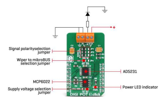
One of its distinctive features is to refresh its wiper register (called RDAC in the device datasheet) after the power on, making it possible to restore the wiper position on power-up, just like the mechanical counterpart. The wiper position register (RDAC) is not
