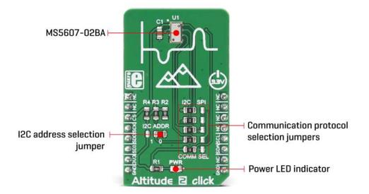
Each sensor IC is factory calibrated at two temperatures and pressures. The calibration coefficients are stored to its 128 bit PROM area. To calculate the correct values, these coefficients need to be used in the calculation, in order to derive real values from the
