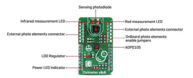
The current from PDs passes through the analog block. The analog block itself contains four AFE signal conditioning sections, which process the input current by using transimpedance amplifiers (TIA) with programmable gain, bandpass filters, and
