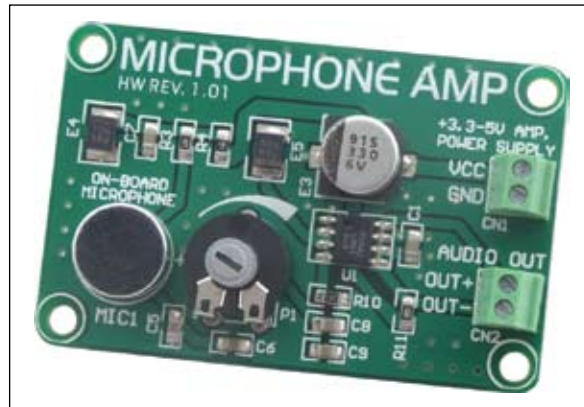
Figure 1: MICROPHONE AMP additional board
