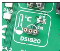
Figure 8-1: DS1820 connector (DS1820 is not placed)
