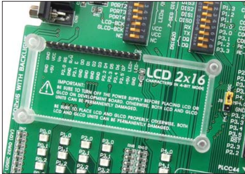
Figure 14-1: Alphanumeric 2x16 LCD display connector
