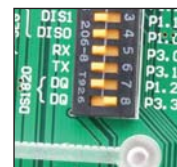
Figure 8-4: Switch 8 on the DIP switch SW8 is in the ON position, DS1820 is connected to the P3.3 pin
