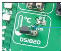
Figure 8-2: DS1820 is plugged into the connector
