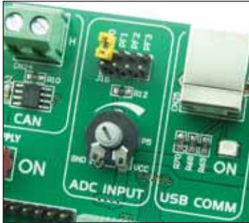
Figure 12-1: ADC (jumper idefault position)
