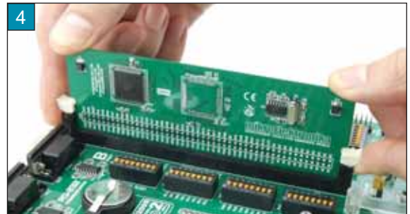
Close the extraction levers when the MCU card is properly placed into the connector
