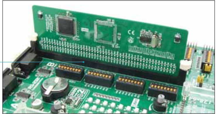
Figure 2-2: DIMM-168P connector with the MCU card inserted
