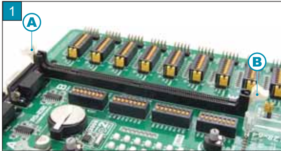
Open extraction levers A and B
