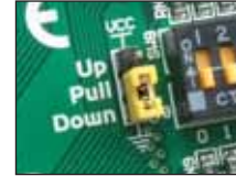
Figure 21-2: J2 in pull-down position
