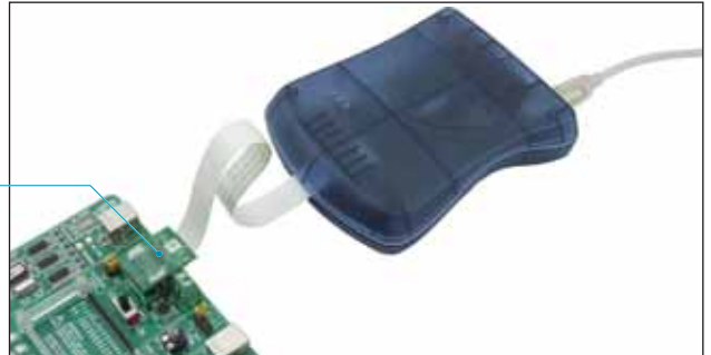
Figure 5-2: JTAGICE mkII connected to the board
