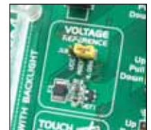
Figure 8-2: Jumper J18 placed to provide 4.096V voltage reference
