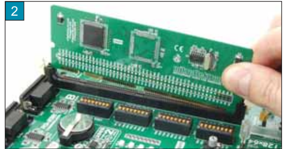
Place the MCU card into the DIMM-168P connector
