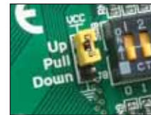
Figure 21-3: J2 in pull-up position
