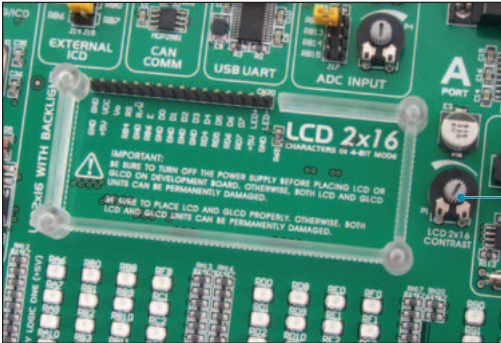
Figure 17-1. Alphanumeric LCD connector
