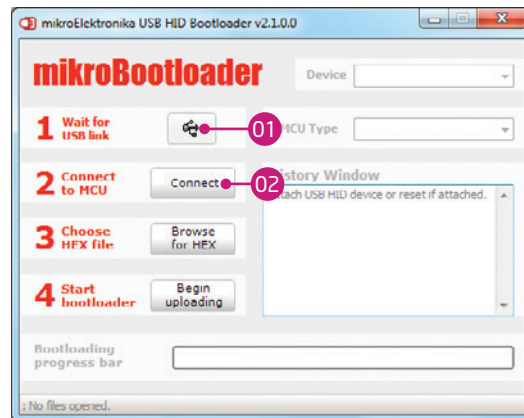
Figure 3-2: USB HID mikroBootloader window
