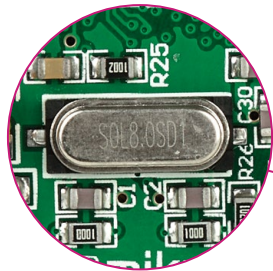
Figure 5-1: External crystal oscillator (X1)
