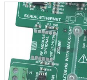
Figure 10-2: Connector for ZigBee module
