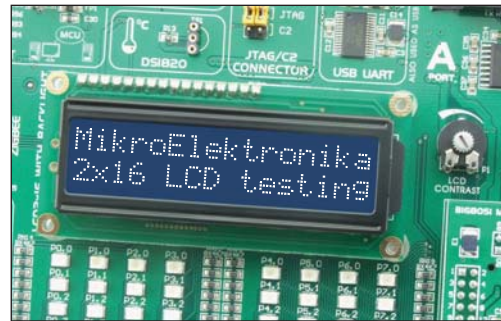
Figure 18-2: Alphanumeric 2x16 LCD display
