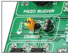
Figure 10-1: DS1820 connector (DS1820 is not connected)
