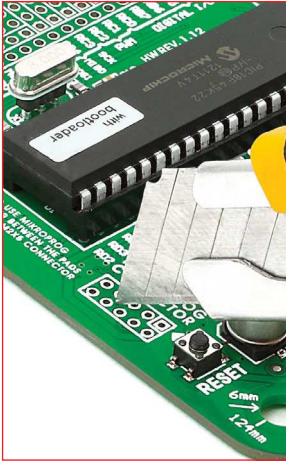
Figure 3-2: cutting copper between pads
