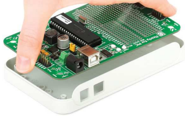
Figure 8-1: Place the board into the bottom part of the casing. Make sure that the connectors are aligned with square openings
