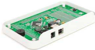
Figure 9-2: Wind screws into inner screw holes to mount the board to the bottom casing plastic
