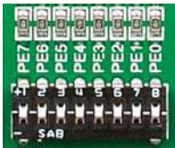
Figure 6-2: Tri-state DIP switch on PORTE
