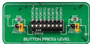
Figure 6-5: Button press level DIP switch (tri-state)
