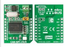
CAN SPI click 5V is an accessory board in **mikroBus**<sup>TM</sup> form factor. It is the best solution for adding CAN connectivity to your microcontroller with SPI interface. Board features **MCP2551** CAN transciever circuit which provides CAN serial communication physical layer in accordance with the ISO 11898 standard. It is designed for operation in especially-harsh environments, providing reliable solution. Board is designed to use 5V power supply only.
