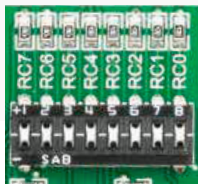
Figure 6-2: Tri-state DIP switch on PORTC
