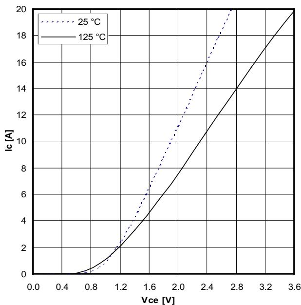
Typical output characteristics,  $V_{GE} = 15$  V
