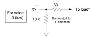
\*Note: Do not use a TTL load. This will overcome the 10 k $\Omega$  pull-down and force the input to a logic 1.
