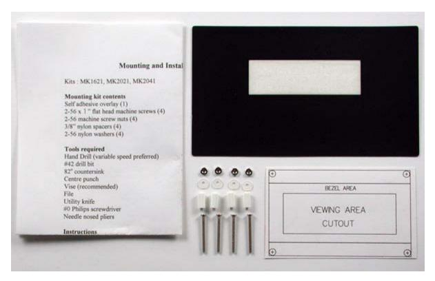
Mount a 20 character x 4 line display, Product # LK/ VK204-25, LK/ VK204-25-USB, GLK12232-25-FGW/WB (NOT -SM) just about anywhere with this kit. Place the self-adhesive overlay on the surface where you'd like to mount the display; use it as a guide for cutting out a window for the display and drilling holes for the mounting screws. Includes: Self-adhesive overlay, adhesive cut and drill guide,
