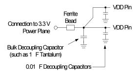
Both VDD pins must be connected to the same voltage.
