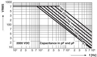
Permissible AC Voltage versus Frequency
