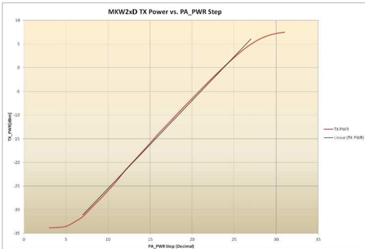
Figure 2. MKW2xD transmit power vs. PA\_PWR step
