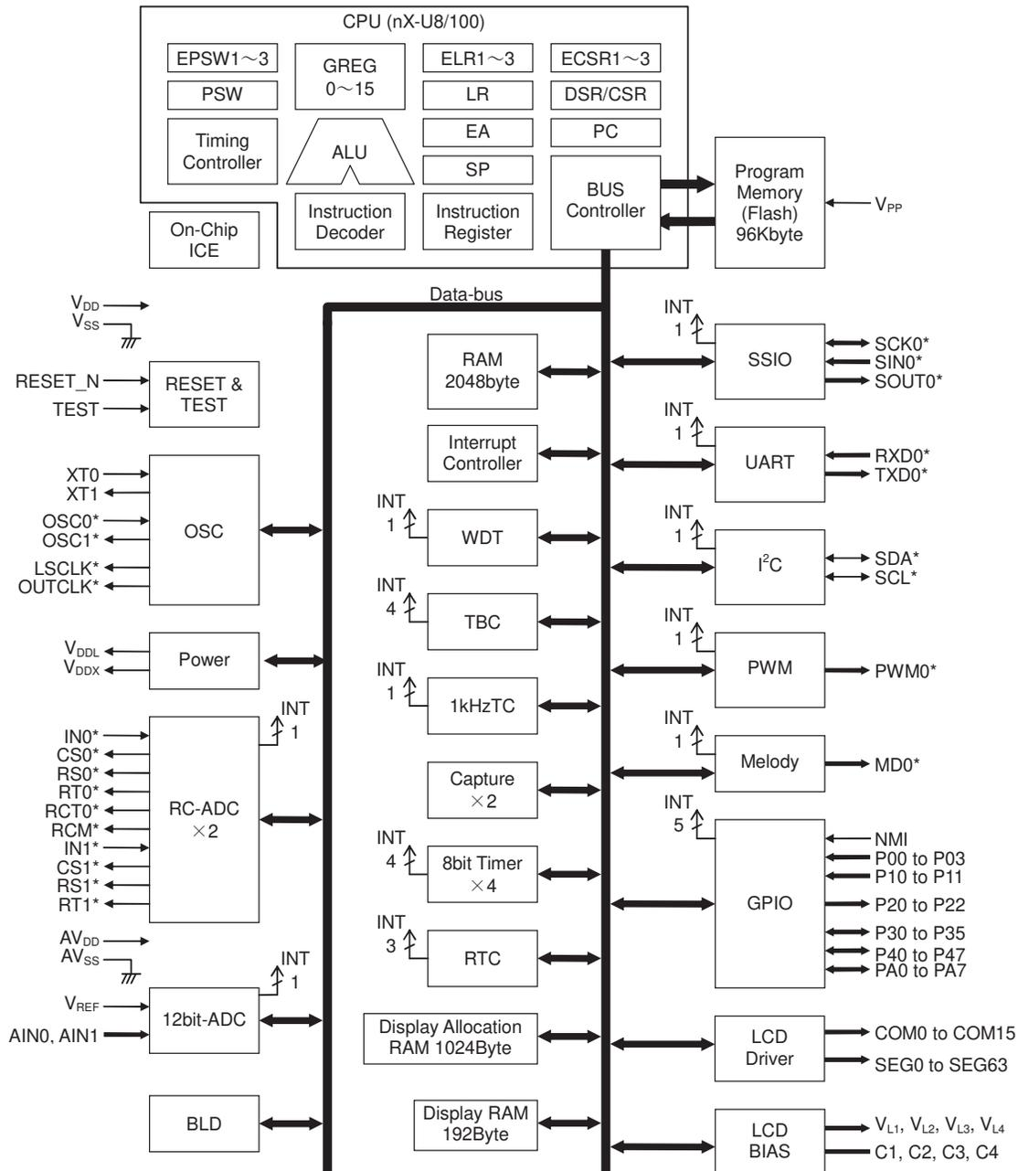
**Figure 1 ML610Q435 Block Diagram**
