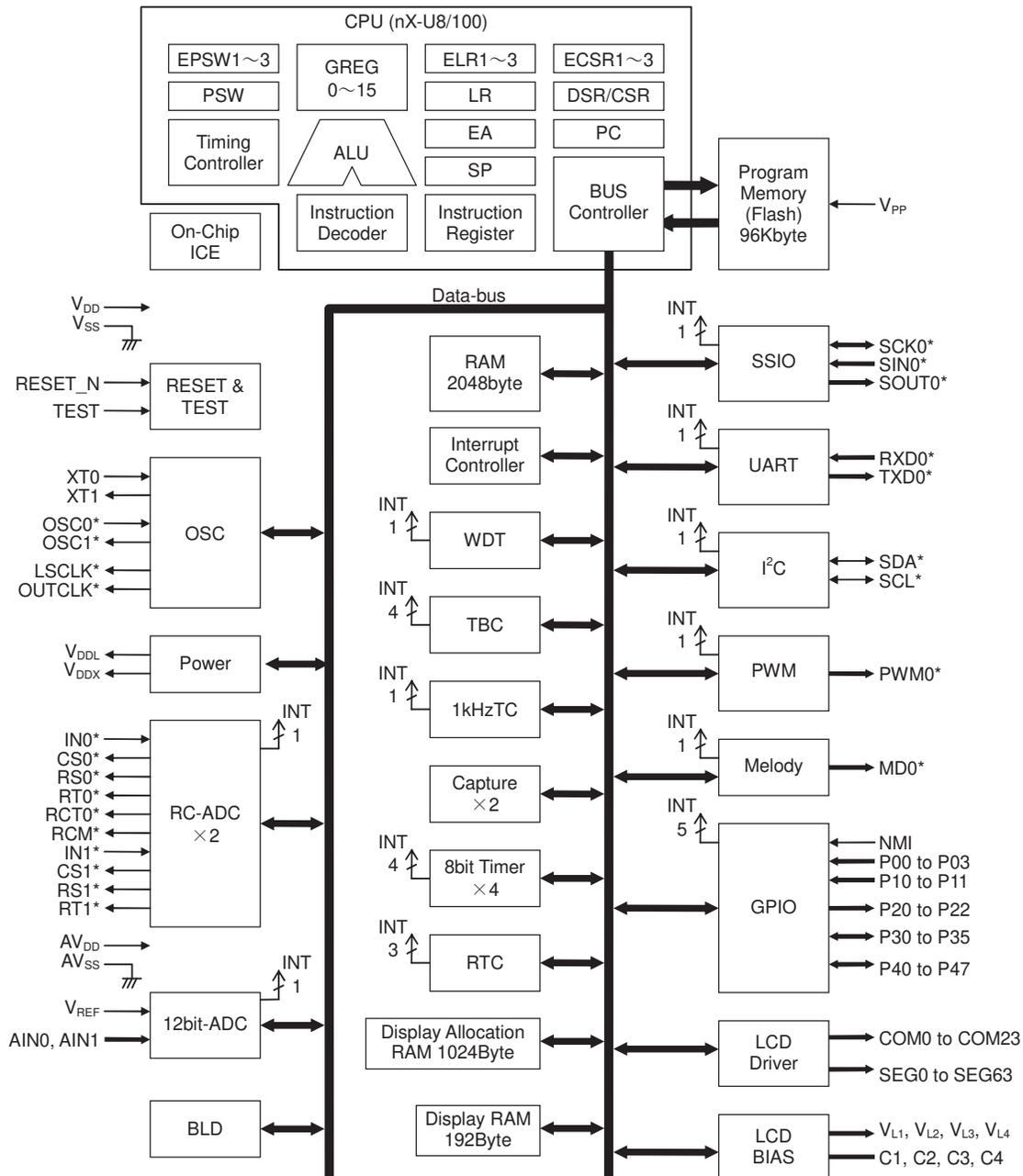
**Figure 2 ML610Q436 Block Diagram**
