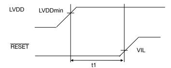
Drive the  $\overline{RESET}$  pin Low and hold it Low under the condition "t1  $\geq$  0[ns]" until LVDD reaches LVDDmin.
