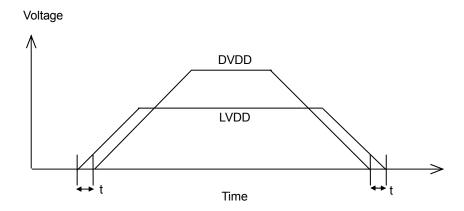
If LVDD is in the range of 0 V to LVDDmin, make sure that LVDD  $\geq$  DVDD and  $t \geq 0$ [ns] are satisfied. When performing power-on reset with a capacitor connected to the  $\overline{RESET}$  pin, be careful about the relationship between the capacitance value and the rise time of the power supply.
