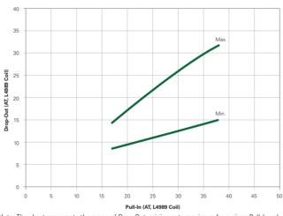
$Note: The \ chart \ represents \ the \ range \ of \ Drop-Out, \ minimum \ to \ maximum \ for \ a \ given \ Pull-In \ value.$
