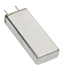
With a profile of 1.0" by 0.5" type MLSG Slimpack capacitors fit into the tightest of spaces and meets a DC test of 5000 hrs at rated voltage, 125 °C. MLSG Slimpack is a perfect fit for military and aerospace applications requiring a low profile, rugged design and long-life. Specify type HRMLSG for high reliability burn-in.
