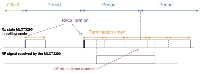
\*The termination timer is postponed as long as a payload is being received.
