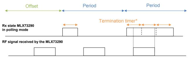
\*The termination timer is postponed as long as a payload is being received.
