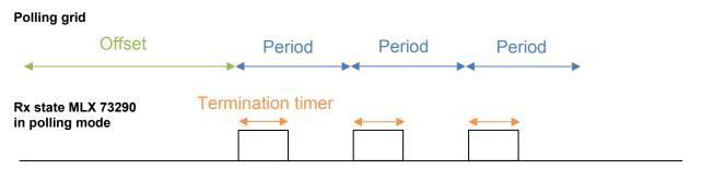
When the timer expires, termination may be postponed while RSSI is above the threshold, or while payload is being received, depending on the setting of the bit RXTERM\_COND. Then the state machine will take the action selected by RXTERM\_ACT: it will stop or recalibrate and resume reception.
