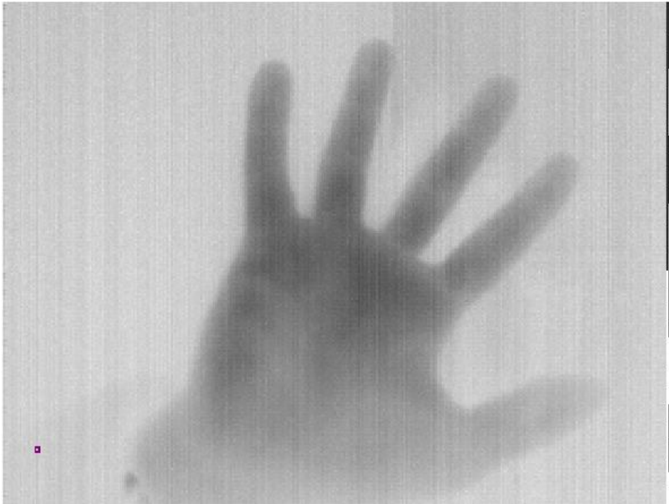
Figure 7: Raw tap A phase0 image of a hand with enabled test columns
