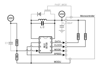
Note: Care should be taken for the capacitor C1 which may reduce the fall time.
