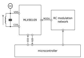
(1): MODE/SPEED config settings (2): DATA/CLOCK outputs
