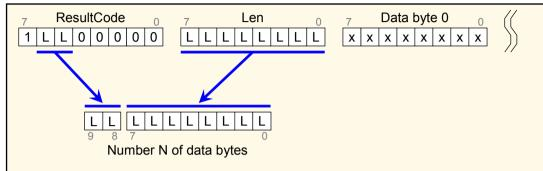
Figure 10: Coding of Length of extended frames
