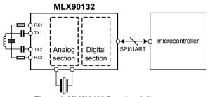
Figure 1: MLX90132 functional diagram
