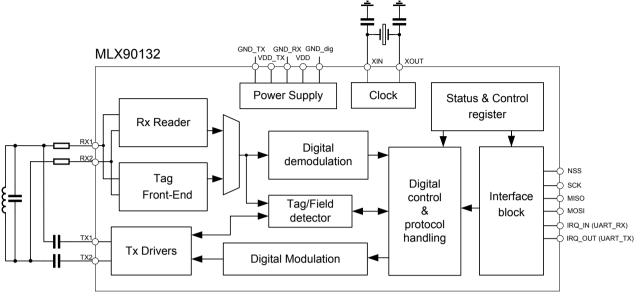
Figure 2: MLX90132 simplified block diagram
