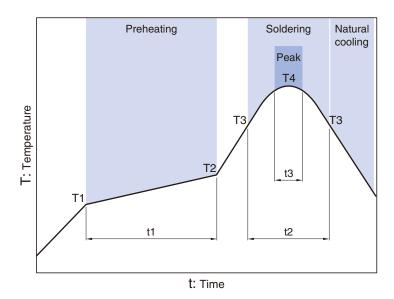
Soldering Preheating Peak Temp. Temp. Time Time Temp. Time T1 T2 T4 t3 Т3 150°C 180°C 60 to 120s 230°C 30 to 60s 250 to 260°C 10s max.
