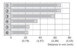
Max. sensing range  $S_n$ , flush or non-flush installation, non-magnetizable material
