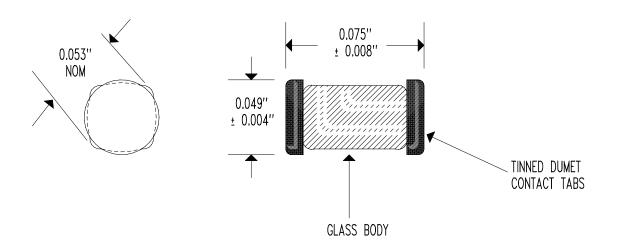
RESISTANCE @  $+25^{\circ}$ C =  $15,000 \Omega \pm 10\%$ RESISTANCE/TEMPERATURE CURVE = "J" BETA " $\beta$ " (0 TO  $+50^{\circ}$ C) =  $3,892^{\circ}$ K NOMINAL TEMPERATURE COEFFICIENT @  $+25^{\circ}$ C = -4.4%/C NOMINAL DISSIPATION CONSTANT = 1 mW/°C NOMINAL THERMAL TIME CONSTANT = 5 SECONDS MAXIMUM MAXIMUM TEMPERATURE RATING =  $+220^{\circ}$ C
