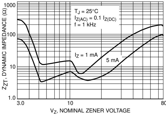
Figure 1. Effect of Zener Voltage on Zener Impedance
