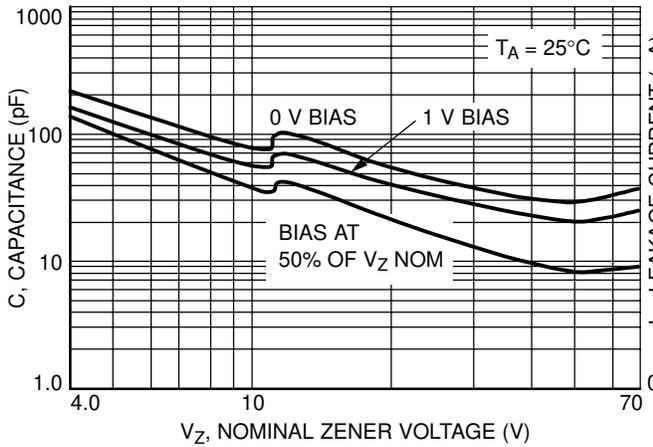
Figure 3. Typical Capacitance
