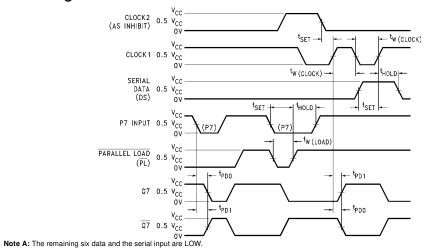
Note B: Prior to test, HIGH level data is loaded into the P7 input.
