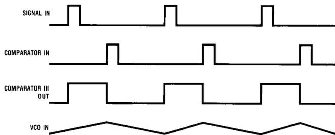
FIGURE 9. Typical Waveforms for Phase Comparator III
