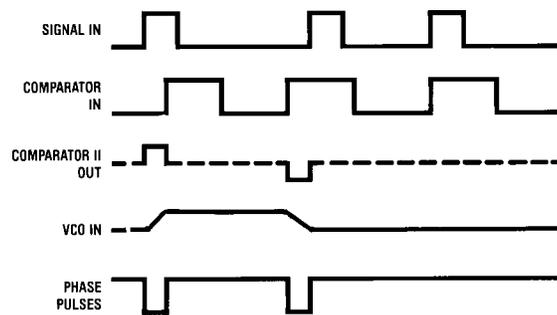
FIGURE 7. Typical Phase Comparator II Output Waveforms
