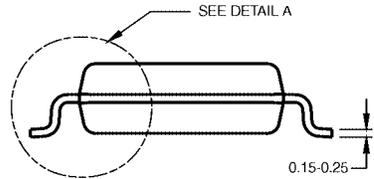
DIMENSIONS ARE IN MILLIMETERS
