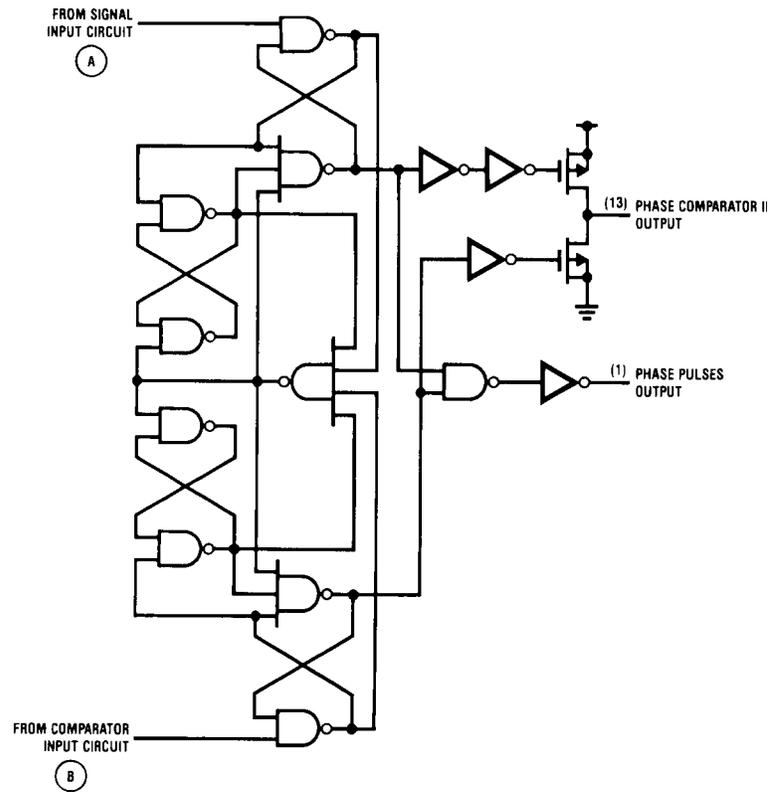
FIGURE 6. Logic Diagram for Phase Comparator II
