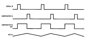
FIGURE 9. Typical Waveforms for Phase Comparator III
