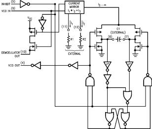
FIGURE 2. Logic Diagram for VCO
