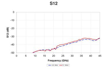
Typical IC performance measured on-wafer
