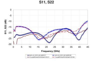
Typical IC performance measured on-wafer
