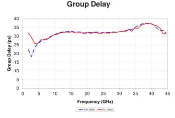
Typical IC performance measured on-wafer
