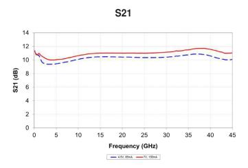
Typical IC performance measured on-wafer
