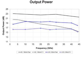
Typical IC performance measured on-wafer
