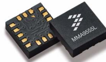
16-pin LGA 3 mm x 3 mm x 1 mm Case 2094-01
