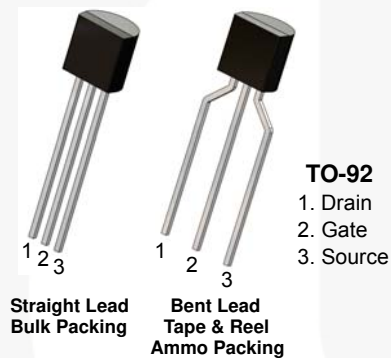
Figure 1. J175 / J176 Device Package
