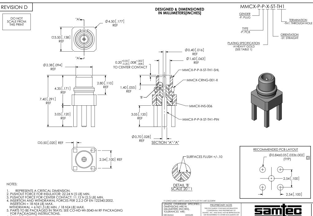
TABLE 1: MATERIAL SAMTEC PART NUMBER ITEM MATERIAL PLATING - (REFERENCE) MMCX-P-P-X-ST-TH1-SHL SHELL BRASS C3604B 0.00013[.000005] GOLD OVER .00127[.000050] NICKEL PTFE TEFLON (WHITE) INSULATOR MMCX-INS-006 N/A MMCX-P-P-X-ST-TH1-PIN PIN BRASS C3602B 0.00076[.000030] GOLD OVER .00127[.000050] NICKEL MMCX-CRNG-001 C-RING BeCu C17300 0.00008[.000003] GOLD OVER .00127[.000050] NICKEL
