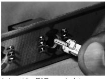
Insert the PWB receptacle/ incandescent lamp assembly through a hole in the printed wiring board.
