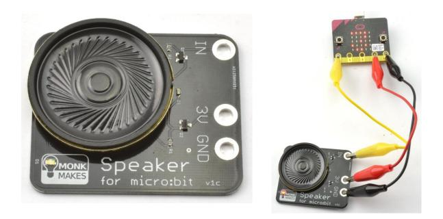
The MonkMakes Speaker for micro:bit is a neat little amplified speaker that connects to your micro:bit using alligator clips.
