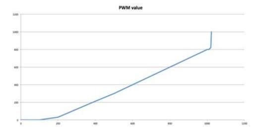
The y-axis shows the current in mA for a test load resistor supplied from a constant voltage source. The x-axis is the analog write value (0 to 1023). As you can see, there is a dead zone up to a analog output value of about 100, followed by a relatively good linear region right up to about 1000, after which the output effectively becomes 'on'.
