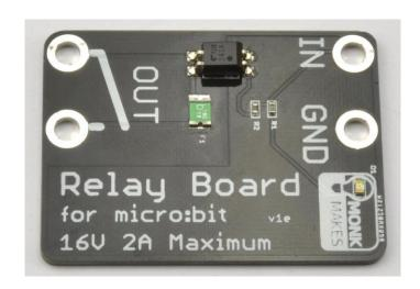
The MonkMakes Relay for micro:bit is a solid-state (no moving parts) relay that allows an output of a micro:bit to turn things on and off.
