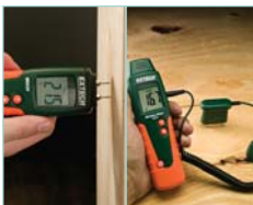
Measure moisture directly on the material or use remote handpress moisture probe (included) on hard materials.
